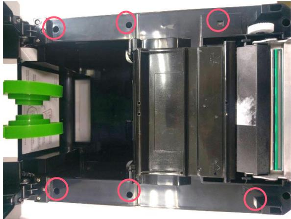
2. Remove the 10 screws on the ribbon base module.
