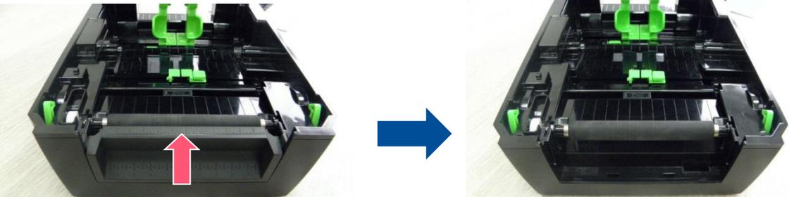
2. Disengage the platen holder tabs by pulling out the right side and left side tabs. Rotate the tabs into the forward position. (see picture below)
