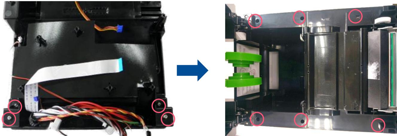
3. Remove 6 screws to remove top cover assembly.
