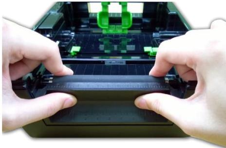
6. Hold the grounding cable onto the right side of the peel-off bar. Then, install the peel-off bar into both slots on front inner lower cover. Please install left side (with spring) first. **Make sure the flat side of grounding wire is on right side as shown below.**
