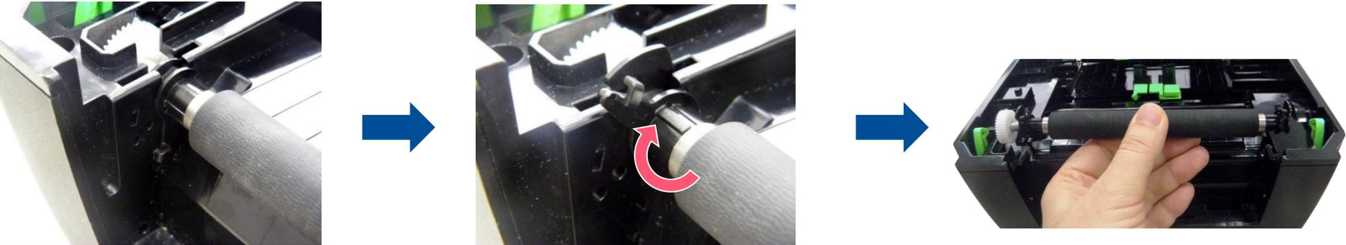
3. Take out the platen roller assembly to replace. Reassemble the parts in the reverse procedure.
