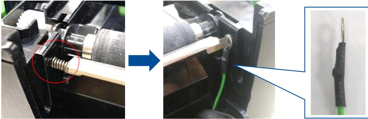
7. Put the peel-off module harness through the slot of the lower inner cover front side.
