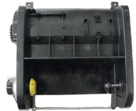
3. Remove/Replace the ribbon base module.
