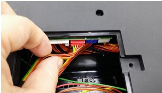
**10.** Hook peel-off module harness and grounding cable onto the printer lower cover. Secure back the printer bottom cover by one screw.
