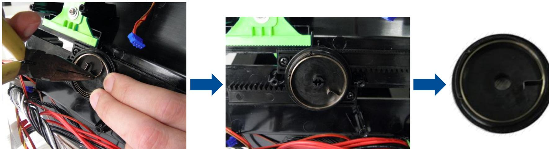
5. Remove four screws to replace the media holder assembly.
