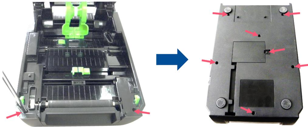
2. After removing the lower cover, remove two screws securing the main board on the lower inner cover. (no need to disconnect all the cables on the main board)
