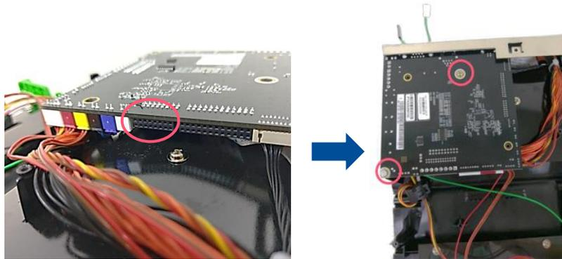
4. Install the wireless interface board into the main board.
