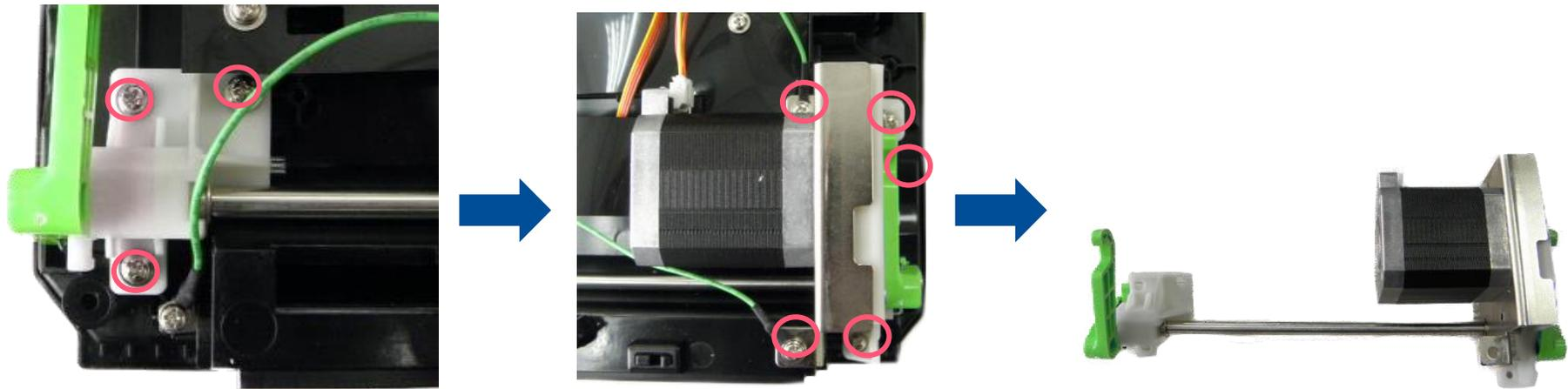
5. Remove one e-ring to replace stepping motor module.
