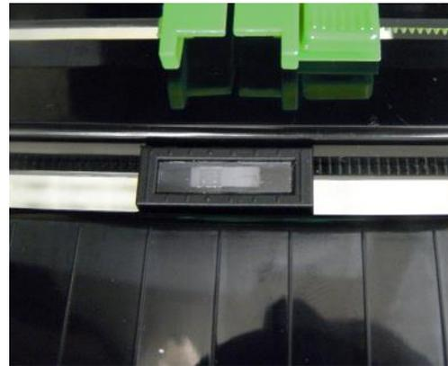
4. Remove/replace the black-mark sensor module.
