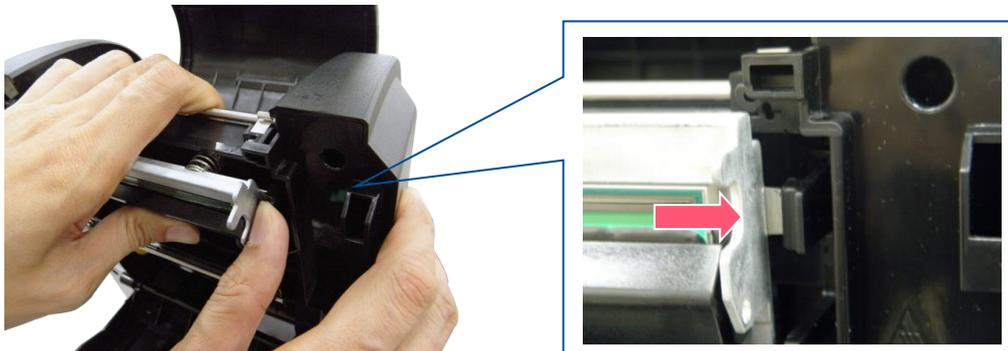
4. Disconnect printhead harness and ground cable to replace the printhead module.
