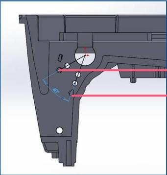
The tab here is for thick label. (Thickness is 0.19 mm)
