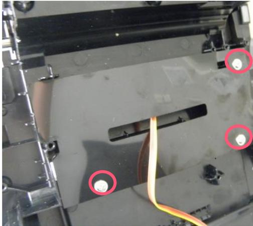
3. Remove two screws on the black-mark sensor fixing plate.
