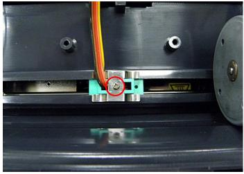
Remove 1 screw on the black-mark sensor fixing plate.
