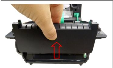
Refer to section 3.2 to remove the lower cover. Open the top cover and pull up the front panel from the printer.
