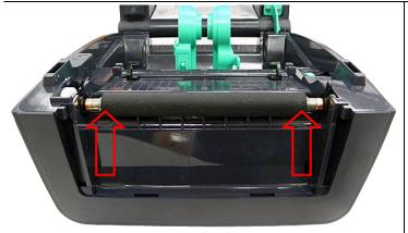
Take out the platen roller assembly and replace a new platen roller assembly.
