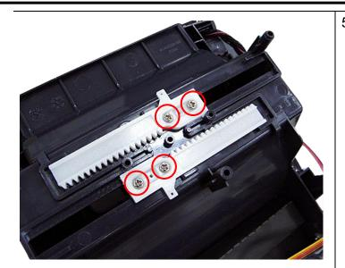
5. Remove 4 screws to replace the media holder assembly.
