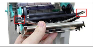
Pull the print head module forward to take out the module and disconnect the print head harness.
