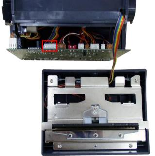
3. Connect the cutter module harness connector to the 8-pin white socket on the printer main board.
