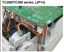
3. Remove 2 screws to replace stepping motor.
