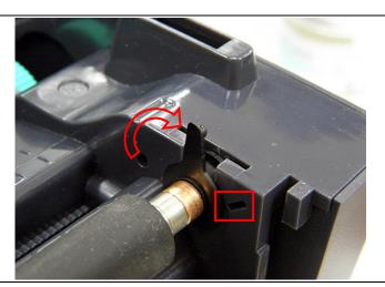
2. Disengage one of platen holder tab from lower inner cover and rotate the tab 90 degrees to install the peel-off bar into the both slots.
