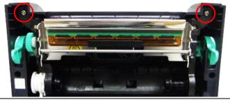
2. Remove 2 screws that hold the print head bracket.
