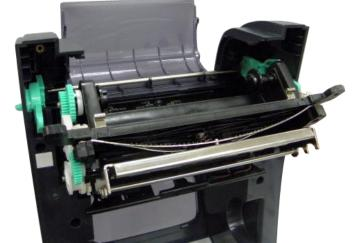
Open the ribbon access cover. Let print head bracket drops into its place.
