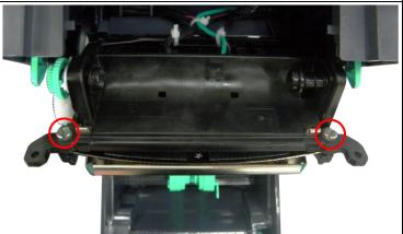
4. Use the slotted screwdriver to remove 2 screws that fix the print head spring plate.
