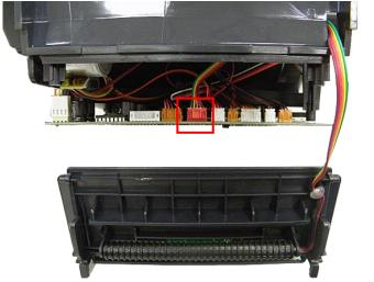
Plug in the peel-off module harness connector to the 5-pin red socket on the main board.
