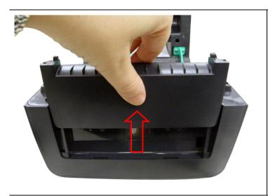
Open the printer top cover to remove the front panel.
