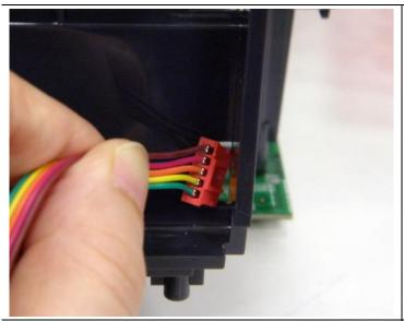
4. Thread the 5-pin peel-off module harness through the front slot of lower inner cover.
