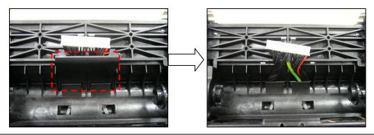
7. Insert the new print head module spring plate into the ribbon base print head spring plate slot. **Make sure the TPH bracket hinge slots are engaged with the hinges at both sides.** Reassemble the parts in the reverse procedures.
