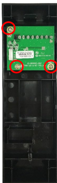
ML240/MA2400C Series LED panel with three screws
