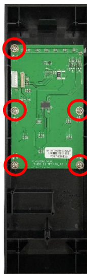
ML240P Series LCD panel with five screws
